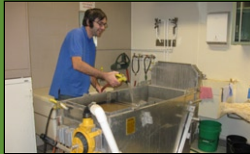
Bryan Kendall working the flotation machine in OSA lab.
